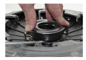
To release the bearing from the cover, apply pressure to the top of the bearing until the bearing moves very slightly downwards and insert a flat head screwdriver in between the bearing and the sprung retaining clip.
